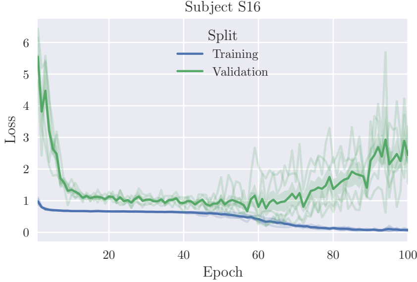
Figure 3.7: Spectrogram-based CNN model optimization: Training and validation loss for all cross-validation folds for a single subject. Thick blue and green lines represent the average over all folds for training and validation, respectively.
